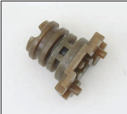
Figure 9: Remove snout from solenoid B and use it to retain the 2-3 shift valve. Leave the O-ring off.
